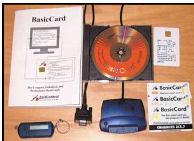
Photo 1 —Check out the development kit. Don't bother unwrapping the CD-ROM. You should download the up-to-date software directly from ZeitControl's web site.
