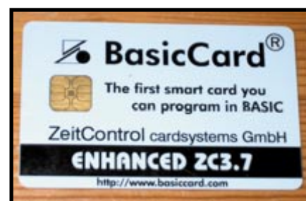
Photo 2 —The BasicCard MCU is under the gold contact area.
