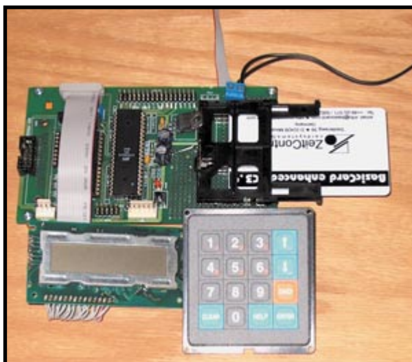
Photo 1—Check out the monitor before it's mounted in its cabinet. Note the BasicCard sticking out of the card socket on the right-hand side.
